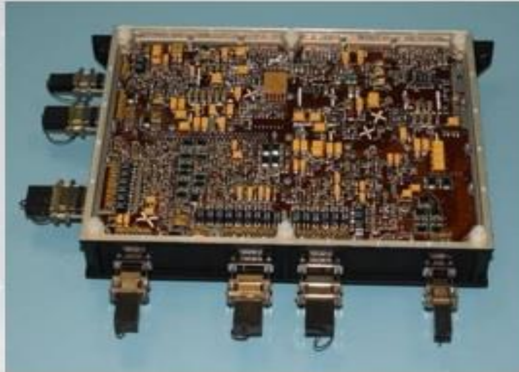
SOLAR ORBITER - RPW LVPS Power Supply Board
