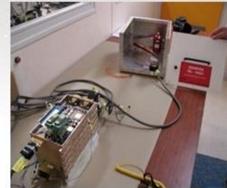
DEMETER - I/V Converter - 2001 I/V Converter for Langmuir Probes pA to \mu A current range to voltage
