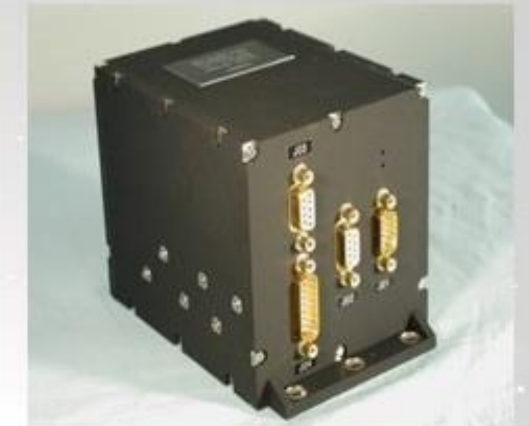
SMART1 - EPDP - 2002 First European Mission to the Moon EPDP Measuring Unit, CAN bus
