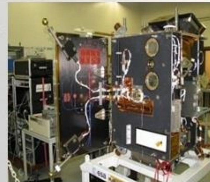
PROBA2 - DSLP&TPMU - 2006 Data Processing & Communication Unit 2x I/V Converters for Langmuir Probes
