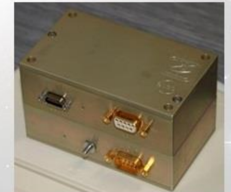
PROBA-V - SATRAM - 2013 Multispectral Earth Observation Time-Pix Radiation Monitor
