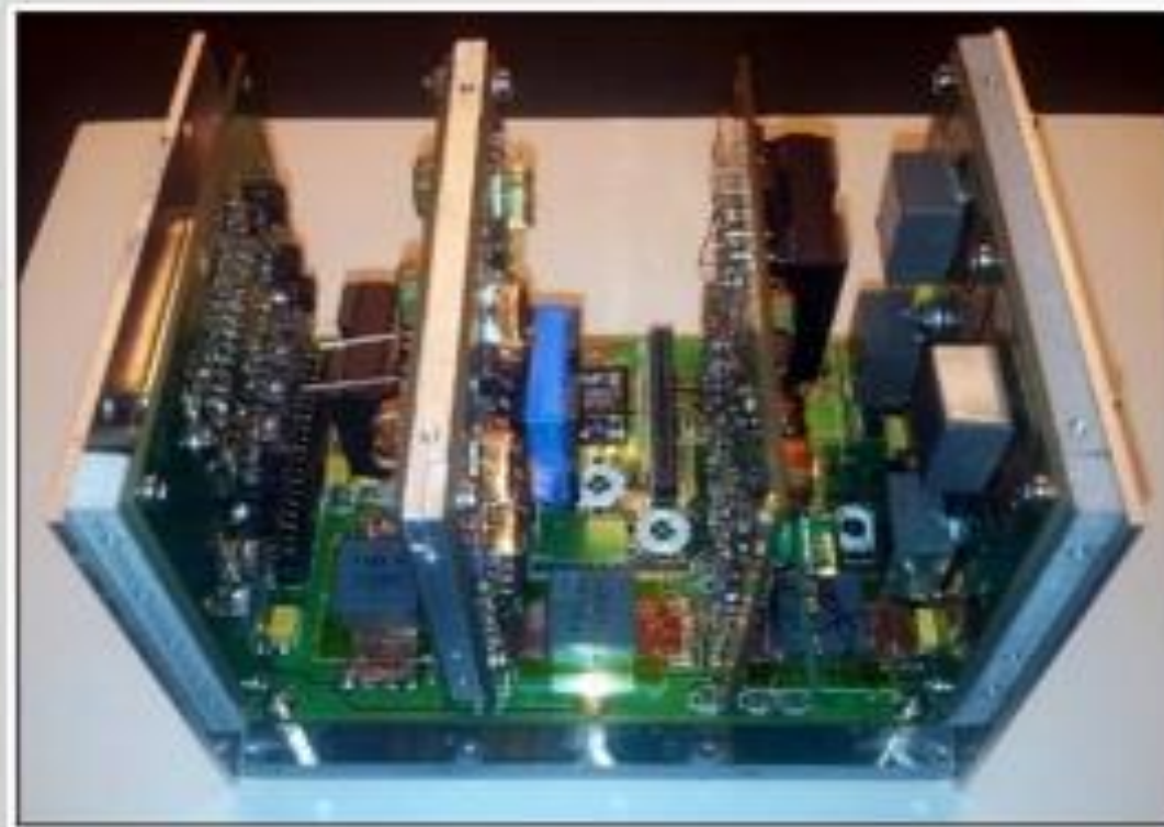
ELISA - PWR Power Supply for Laser Head
