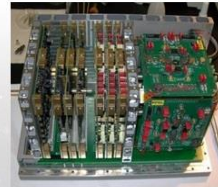
SWARM - MAC - 2011 Microaccelerometer PWR, DPU, Sensor Units
